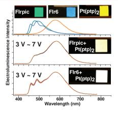
Undoped yellow-orange and white OLEDs based on a Pt(II)-phosphor [Pt(ptp)<sub>2</sub>] realize very high power efficiencies of  $79.2 \pm 0.2 \text{ Im W}^{-1}$  and  $49.5 \pm 0.1 \text{ Im W}^{-1}$ , respectively. The working mechanisms of both devices are studied to unveil the determining factors leading to such high efficiencies.
