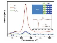
Hybrid interface states and spin polarization are observed at ferromagnetic metal (FM)-organic interfaces, which result from the chemical interaction and hybridization between the FM and the organic molecules. It provides a way for spinterface engineering in organic spintronics. This approach allows full control of the spin band appropriate for carrier injection, opening up new spintronic device concepts for future exploitation.
