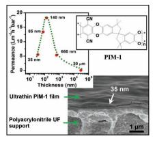
Ultrathin PIM-1 membranes are fabricated and applied to organic solvent nanofiltration. A 140 nm thick PIM-1 membrane shows a permeance value for heptane 90 times higher than Starmem240 (a commercial polyimidebased organic solvent nanofiltration membrane). Its mechanical response is found to be robust to nanofiltration pressures of about 10 bar. The performance of even thinner membranes deteriorates due to enhanced packing upon further confinement.
