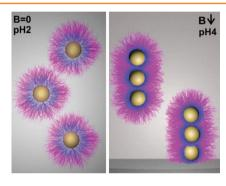
A methodology of making anisotropic, reversibly reconfigurable and erasable coatings is developed. The core-shell superparamagnetic particles with a locking behavior are employed to make the colloidal aqueous dispersion sensitive to pH. Particles are reversibly locked in chains by adjusting pH of the aqueous solution. The anisotropy of the coating is imposed by the external magnetic field.
